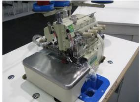
2 needle 4 thread Speed Dry Overlock machine with pneumatic thread chain trimmer and self cleaning system High Speed for better productivity + Dry Finish for less downtime
