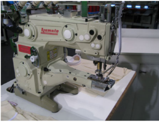
Feed-Up-The-Arm- Interlock Stitch Machine prepared for attaching tape Shoulder-to-Shoulder
