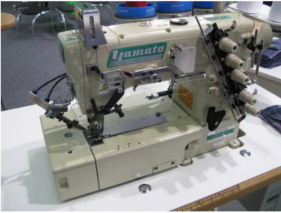
3 Needle- 5 Thread Flatbed Interlock machine with Thread cutters and StitchLock System
