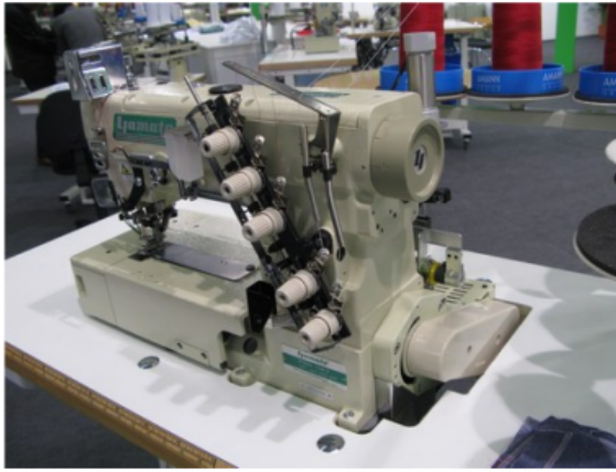
3 Needle- 5 Thread Flatbed Interlock machine with Thread cutters and StitchLock System
