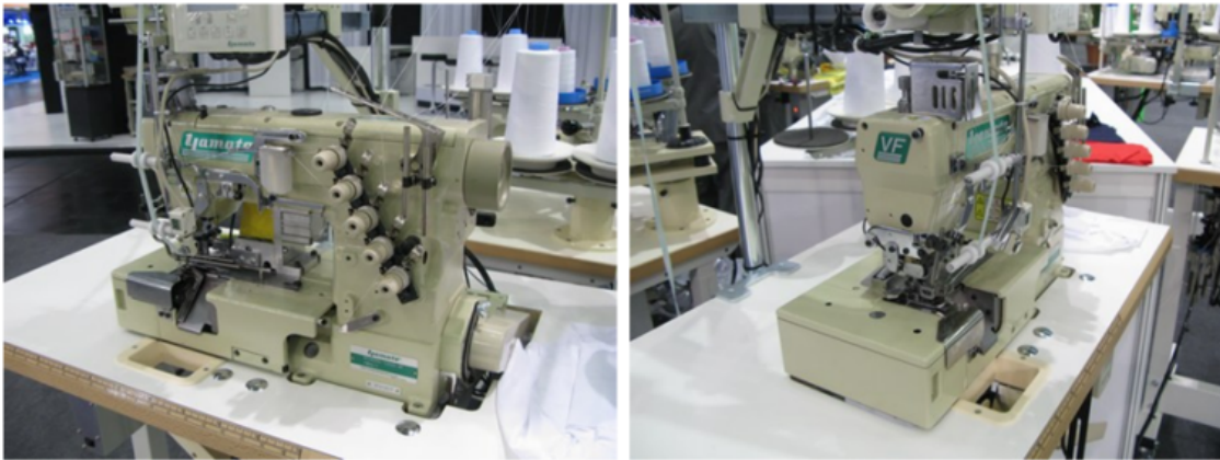
2 Needle 4 Thread Flat Bed Interlock Stitch Machine for Attaching Lace, with Right Hand Fabric Trimmer and Yamato "ACCU-10" Computerized accurate tape tension controller
