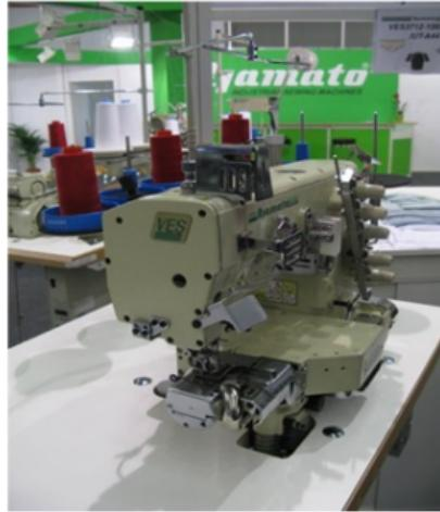
**Extra Small Cylinder Arm Top feeder is available now with Left Knife Fabric Trimmer**
