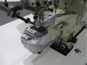
"Streamline" Cylinderbed Interlock Stitch Machine with Active Thread Control and Stitch Locking Thread Trimmer
