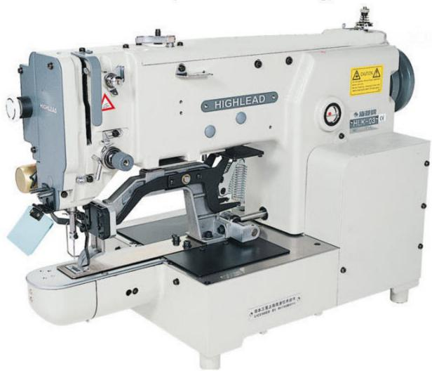
Highlead HLK-03EBS electronic lockstitch button sewing machine programmed to sew two or four hole flat buttons.
