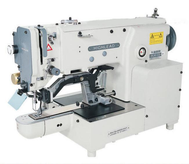
Highlead HLK-03BT electronic bartack sewing machine with 16 different pre-programmed patterns to suit most standard bar-tacking operations.
