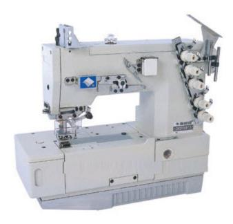
The GK31058-3 is a high speed cover seam (seam-cover) machine from Highlead.
