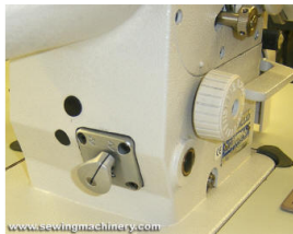
Change over lever fitted with-in machine arm
