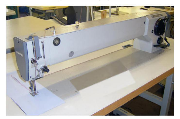
The Highlead GG0028-73L is an extra long arm Zigzag machine designed for use with medium & mediumheavy weight materials.
