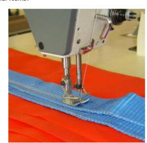
A wide range of sewing threads can be used, with this model being able to sew with up-to size 20 synthetic thread (or size 30 cotton thread) + V69, V92 & V138 heavy duty threads etc.
