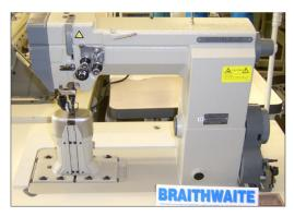
The Highlead GC24618-1 is a twin needle lockstitch post bed machine which features a combined triple feeding system utilizing: needle feed, bottom driven roller feed and top driven roller feed for optimum feeding parformance.
