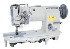
The GC20638 is the twin needle version of Highlead's latest model of heavy duty compound feed lockstitch machine which features a very useful selectable split needle bar.
