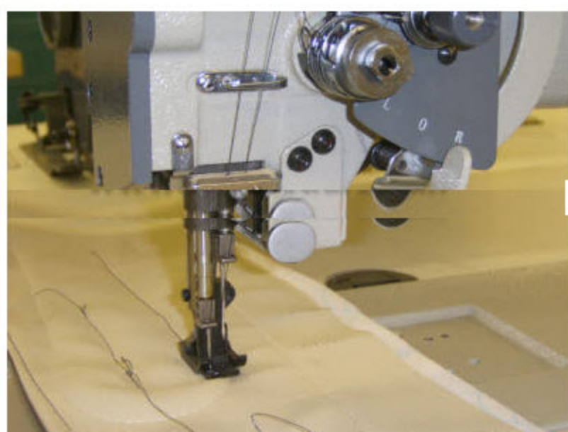
Right needle bar disengaged (lever set to R)
