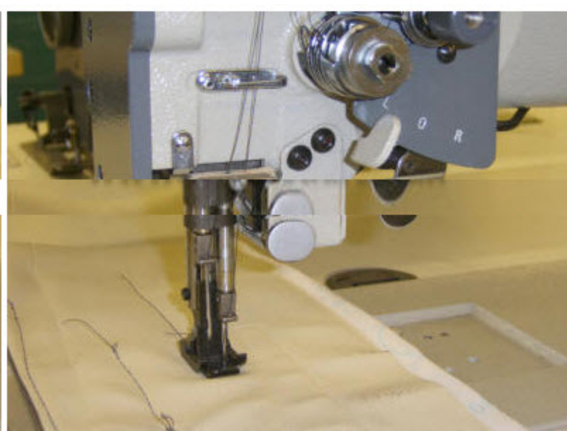
Left needle bar disengaged (lever set to L)
