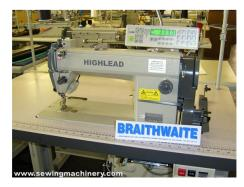
The Highlead GC128-MD3-106 is a single needle lockstitch machine with thread trimmer for use on light/medium weight materials.
