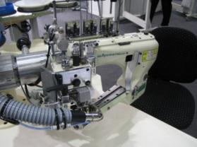
4 needle 6 thread Feed-off-the-arm Both Cut Flatseamer with "Magic DRY" technology (with Air-operated Automatic Chain Cutter)
