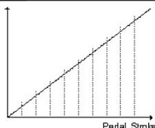
※ Items No. 1~5 : Equal division of pedal stroke in 64 steps, The speed curve of the pedal stroke changes according to how many steps are set up for the divided pedal stroke of each forward pedal step. (Used when adjusting pedal sensor)
