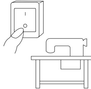
3. Turn off the power when servicing the servomotor or changing the needle.
