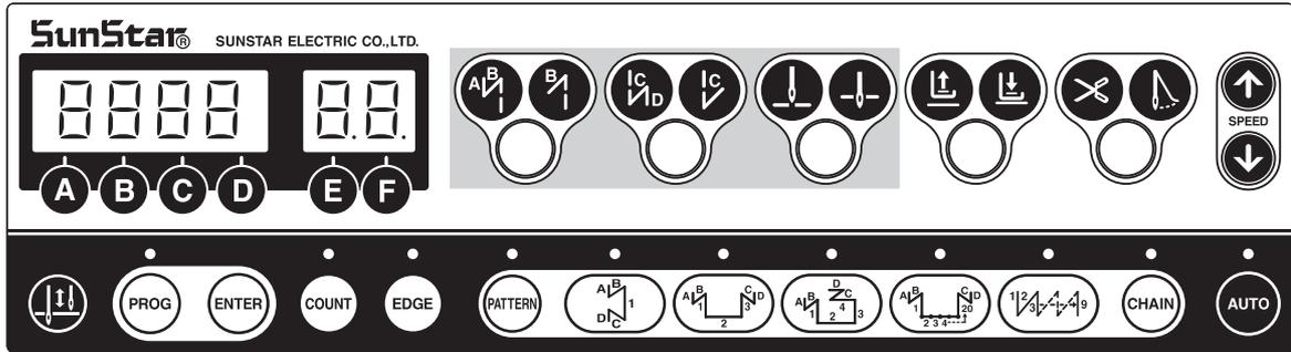
Method of initializing: Turn the power on by simultaneously pressing the buttons in the figure above which are the start B/T button + end B/T button + needle plate up/down stop button.
