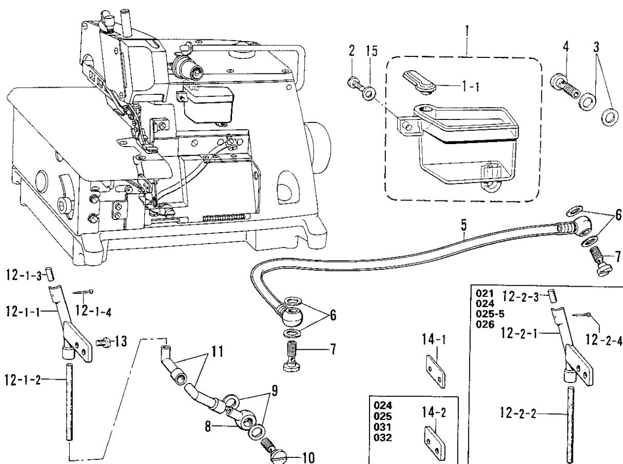
B. 駆動軸関係/Crank shaft mechanism/Kurbelwelle/
