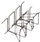
STITCH TYPE 512 FOUR THREAD OVEREDGING
